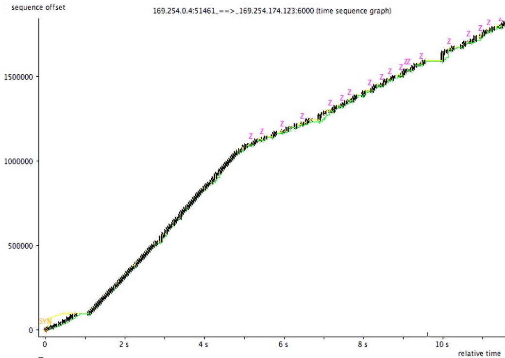
At various points on the overview plot, visual ‘sags’ in the straight line are evident. Given that this is a three-minute trace, any anomalies large enough to be visible at this scale indicate severe problems. Zooming in on any part of the trace reveals countless smaller ‘mini-sags’ indicating that the network was constantly having trouble keeping up with required data rate.
