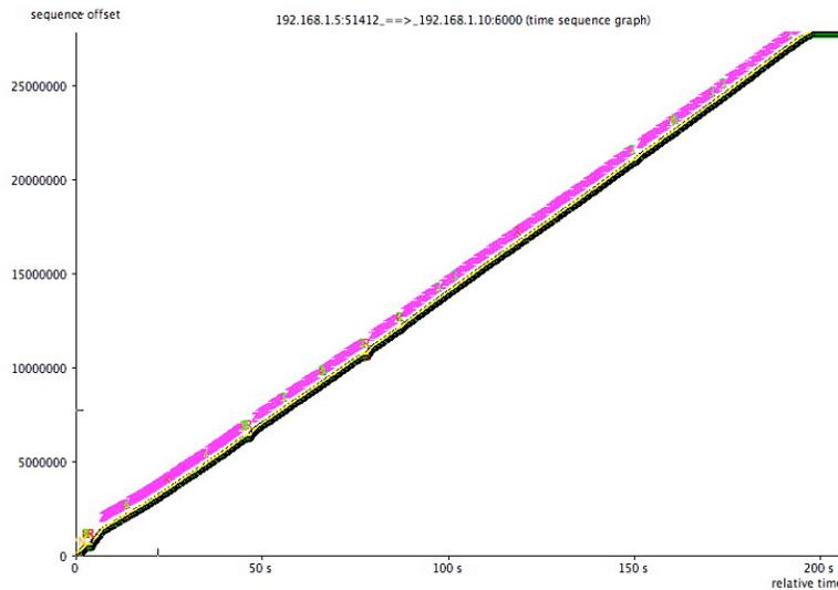
In particular, there was a glitch during the initial buffer filling. This is the kind of event that would cause problems for any device that optimistically decided to start playback before it had built up its full playback buffer:
