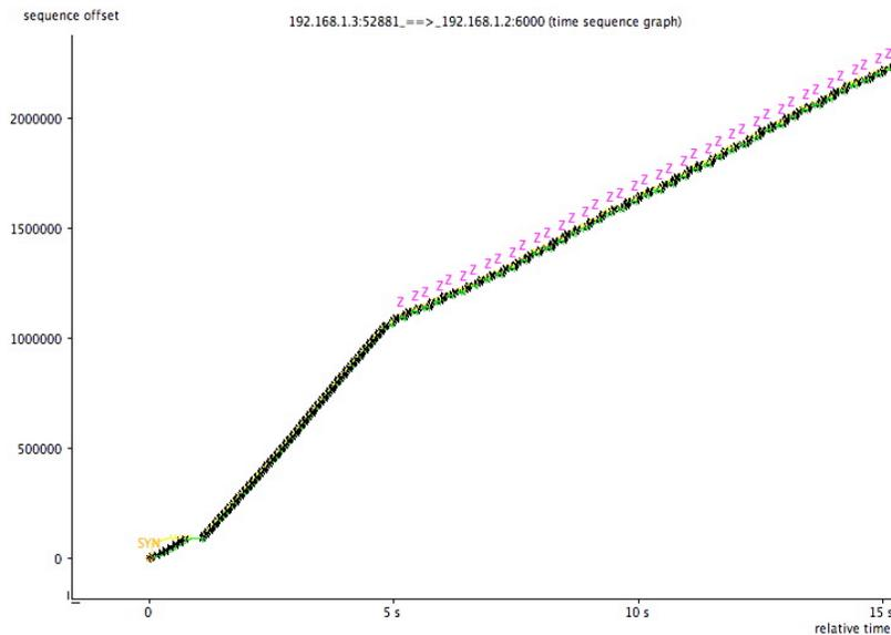
Tcptrace reported no retransmitted packets. Counting only full-sized non-retransmitted TCP segments, the minimum, average and maximum round-trip times reported were: 1.2, 49.7, 120.1 ms, with a standard deviation of 22.2 ms.
