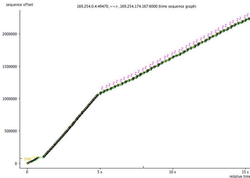
Tcptrace reported no retransmitted packets. The minimum, average and maximum round-trip times reported were: 19.7, 46.2, 105.7 ms, with a standard deviation of 15.9 ms.
